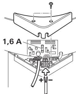
The fine-wire fuse must only be replaced by a fuse of the same design. 1.6 A (slow-acting), EN 60127-2-3.
