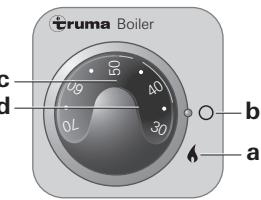
a = Rotary switch "On (Gas operation)"
