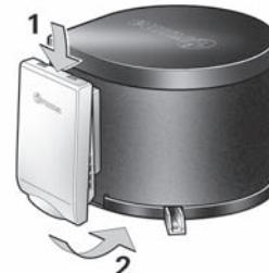
Before every journey, put on the cowl cover when the boiler is switched off. Please ensure that it is secure and has locked into place (risk of accident). Defective cowl caps must not be used.
